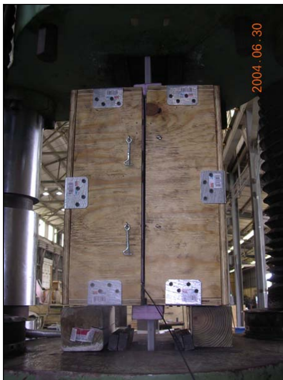
Figure 4.20: Temperature Chamber Surrounding Specimen in 600-Kip UTS
