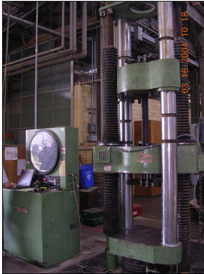
Figure 4.15: 600-Kip UTS Used for Tensile Testing
