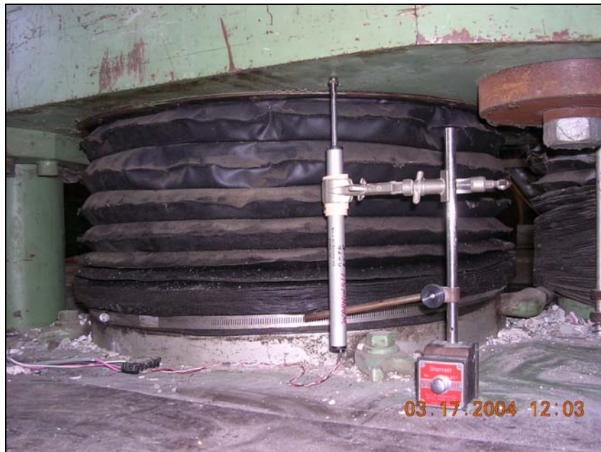
Figure 4.18: Linear Potentiometer Used for Tensile Testing
