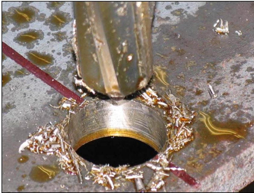
Figure 4.14: Close-Up of Reamer Bit and Hole in Specimen
