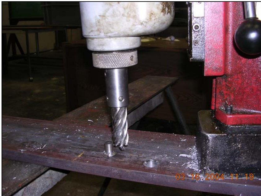
Figure 4.2: Close-Up of Drill, Bit, Slug, and Specimen during Preparation
