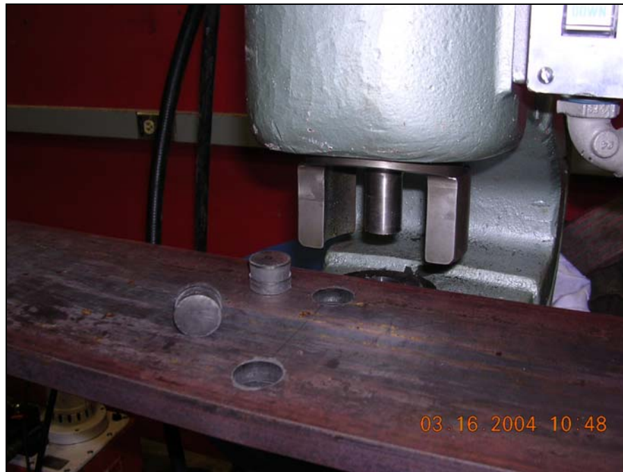
Figure 4.6: Plate and Punched Holes Following Typical Specimen Preparation
