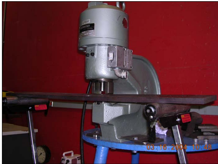
Figure 4.5: Plate Inserted in Punch Press
