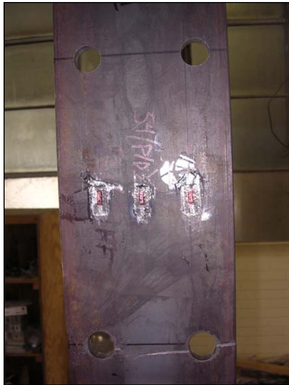
Figure 5.9: Punched and Drilled Fatigue Specimen
