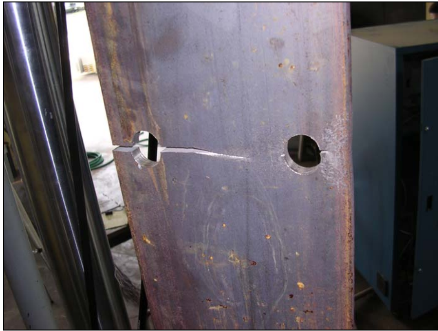
Figure 5.10: Typical Failed Fatigue Specimen
