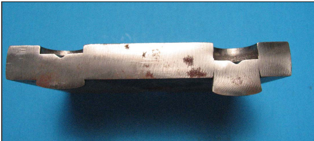
Figure 2.4: Punch Progression at Different Distances through Material (15/16 Inch Diameter Hole in 3/4 Inch Thickness Grade 50 Plate)
