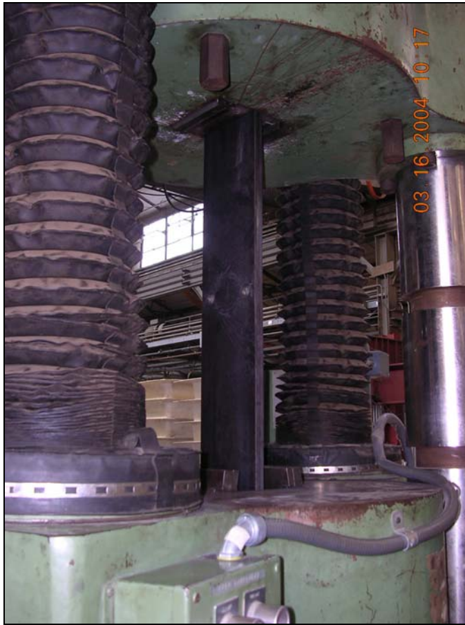
Figure 4.16: Test Specimen in Grips of 600-Kip UTS
