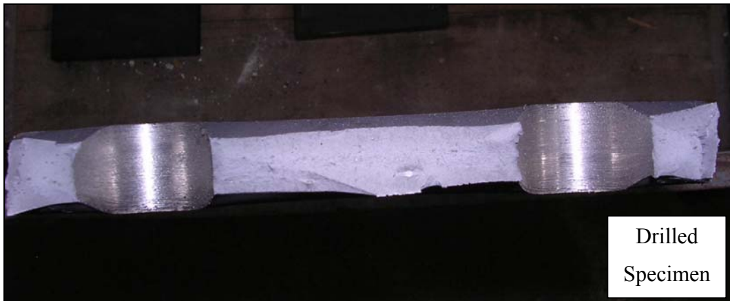
Figure 5.5: Typical Punched and Drilled Hole Fracture Cross-Sections (3/4 Inch Thickness, 15/16 Inch Diameter Hole, Grade 50)
