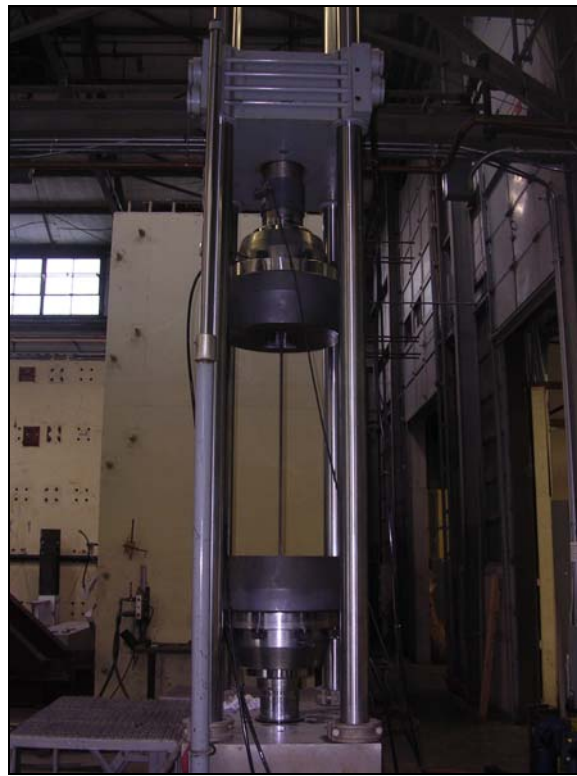
Figure 4.22: Profile of 220-Kip MTS Used for Fatigue Testing
