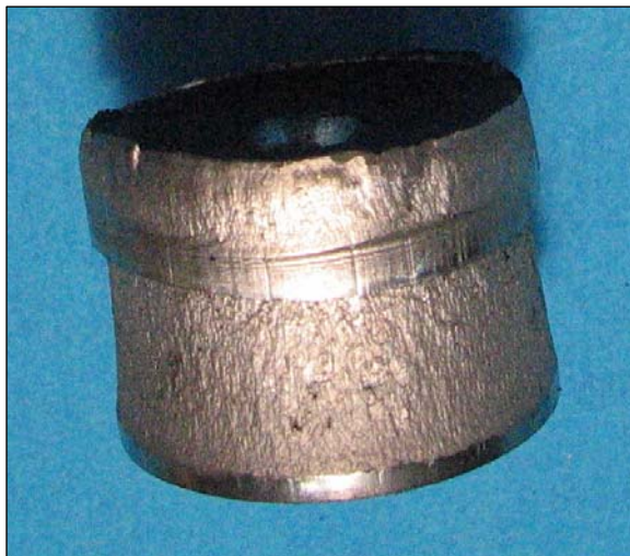
Figure 4.11: AIW Typical 15/16 Inch Diameter, 1/2 Inch Thickness and 15/16 Inch Diameter, 3/4 Inch Thickness Punched Holes (Grade 50)
