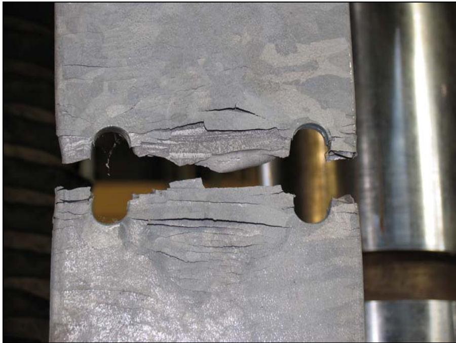
Figure 5.8: Typical Failure of Galvanized Specimen
