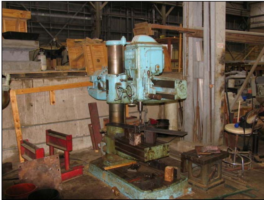
Figure 4.12: High Speed Radial Drill and Reamer
