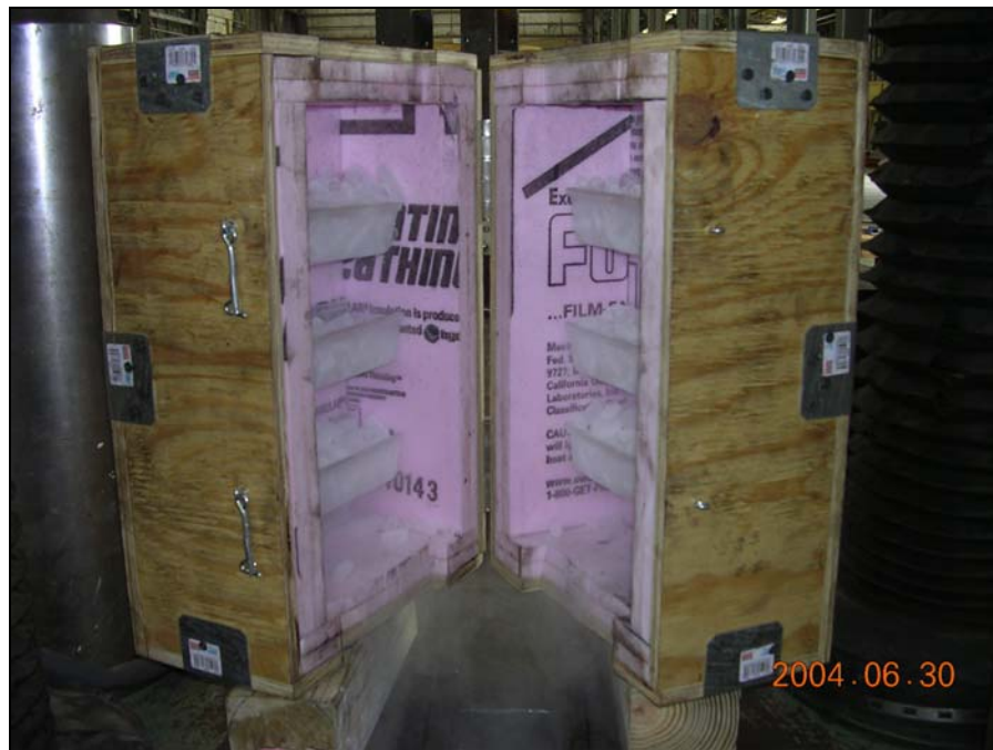
Figure 4.21: Open Temperature Chamber Prior to Tensile Test
