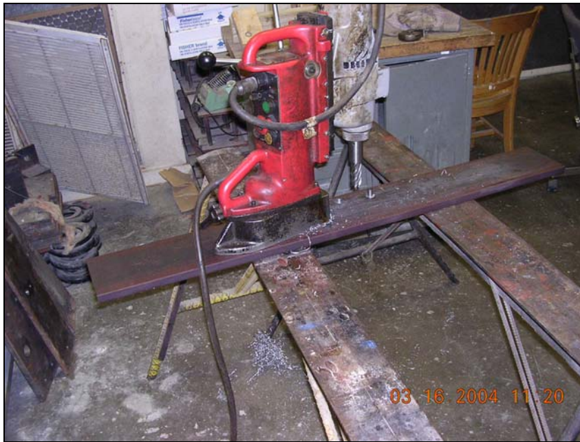
Figure 4.1: Typical Drilled Hole Preparation (with Slugger)
