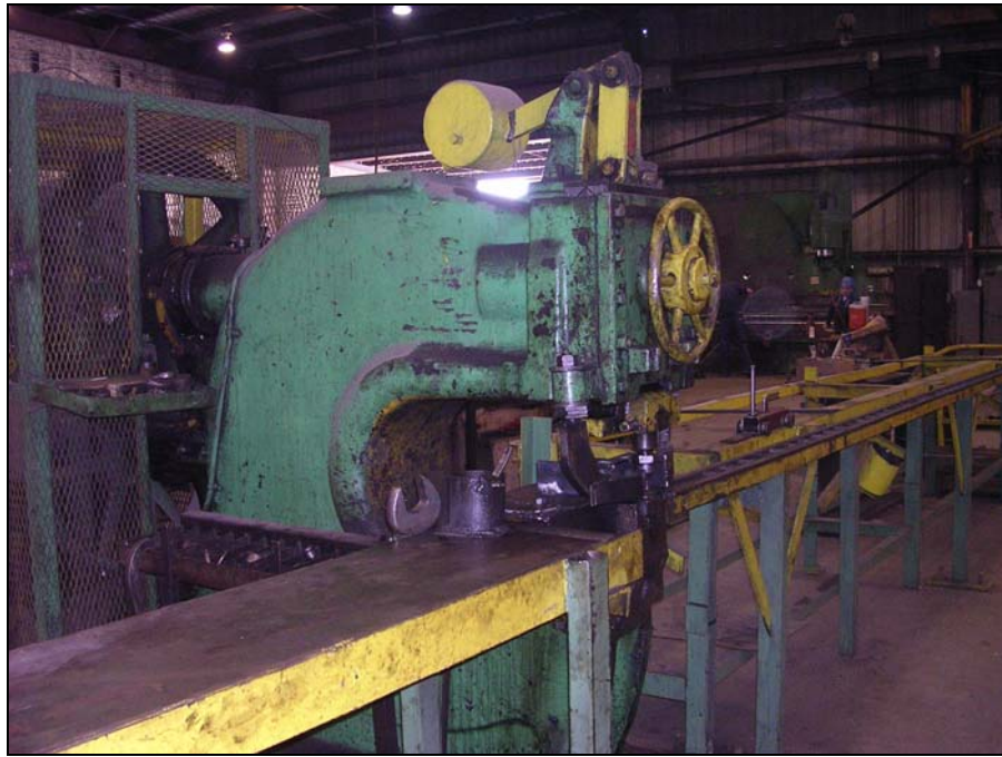
Figure 4.7: Mechanical Punch Press at AIW
