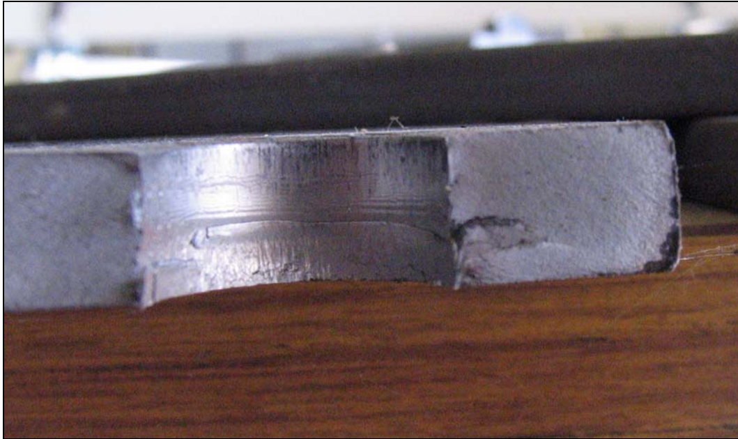
Figure 5.12: Close-Up of Fatigue Crack Fracture Surface
