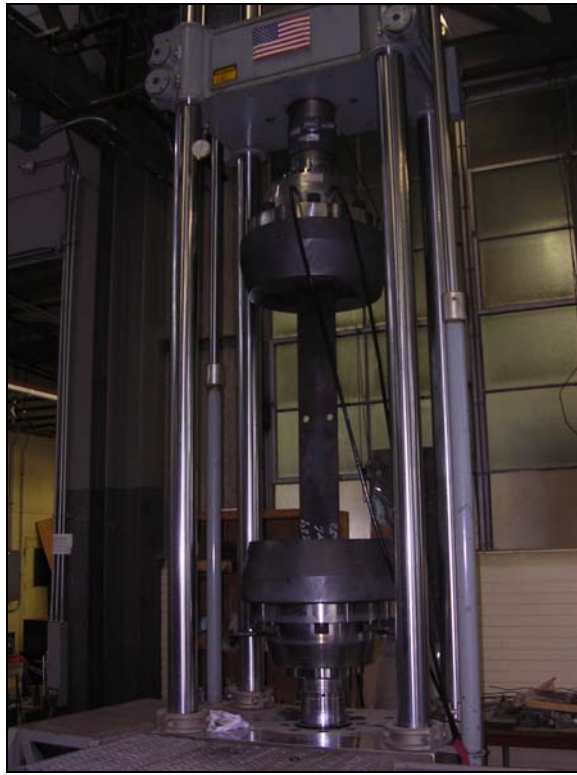
Figure 4.23: Typical Specimen in Grips of 220-Kip MTS
